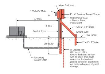
NOTE: Standard Temporary Construction Service in an underground facility is available within 10 feet of existing power facilities (padmount transformers or underground pedestals).
